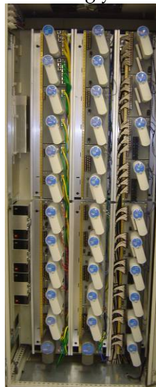
Series C I/O & Controllers Feature a Unique New Vertical Mounting Form Factor That Allows for Smaller Footprint and Improved Thermal Management
