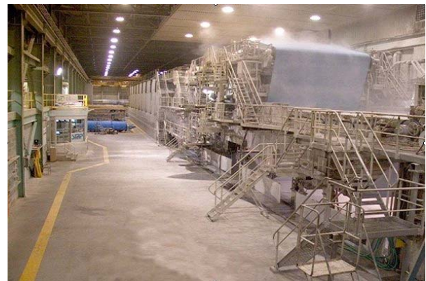
Paper machine 5, St. Marys’ largest producer, supplies paper to supercalenders 5, 6 and 7.
