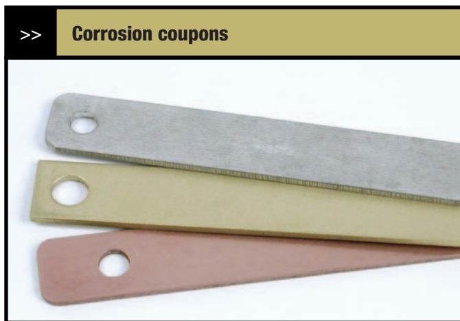
Figure 1. Such coupons continue to play an important role in off-line, retrospective analysis of corrosion.
