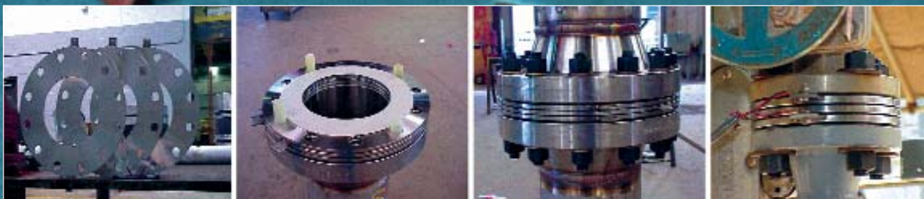
Figure 2. Installation of probe electrodes and electrode insulators in standard ANSI pipe flange.
